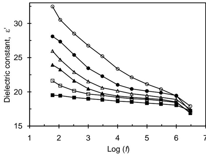
**Fig. 3:** Frequency dependence dielectric constant as a function of temperature for zirconium dioxide. Symbols are used as in Fig. 1.
