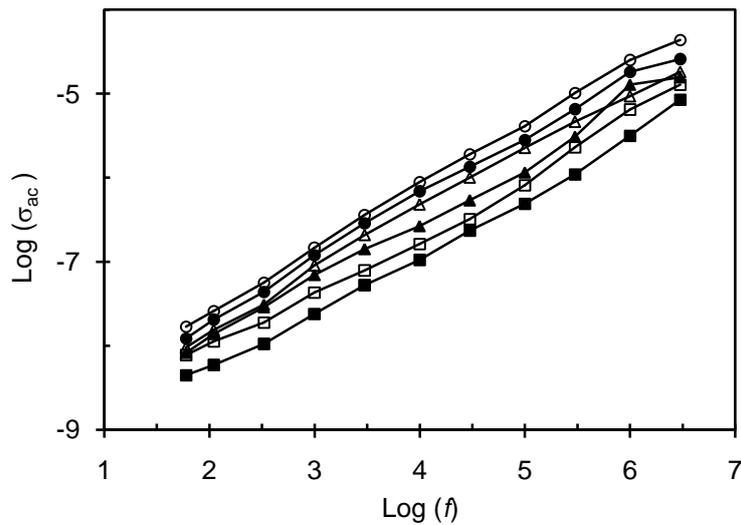
**Fig. 1:** Frequency versus ac conductivity curves aging at; (■) 25, (□) 100, (▲) 150, (Δ) 200, (●) 250 and (○) 300°C for zirconium dioxide.
