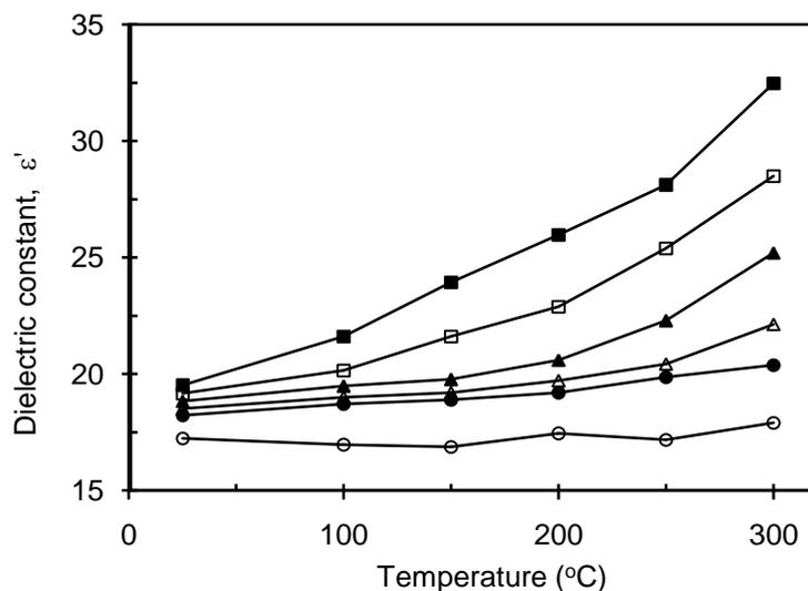
**Fig. 4:** Temperature dependence dielectric constant as a function of frequencies for zirconium dioxide. Symbols are used as in Fig. 2.
