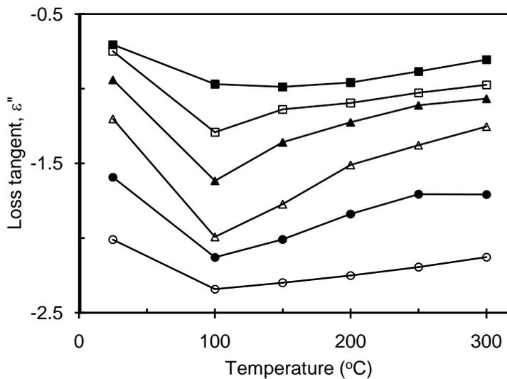
**Fig. 6:** Temperature dependent loss tangent curve as a function of frequency for zirconium dioxide. Symbols are use as in Fig. 2.
