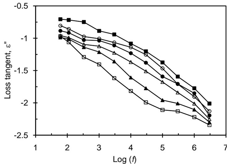
**Fig. 5:** Frequency dependence dielectric loss tangent as a function of temperature for zirconium dioxide. Symbols are used as in Fig. 1.
