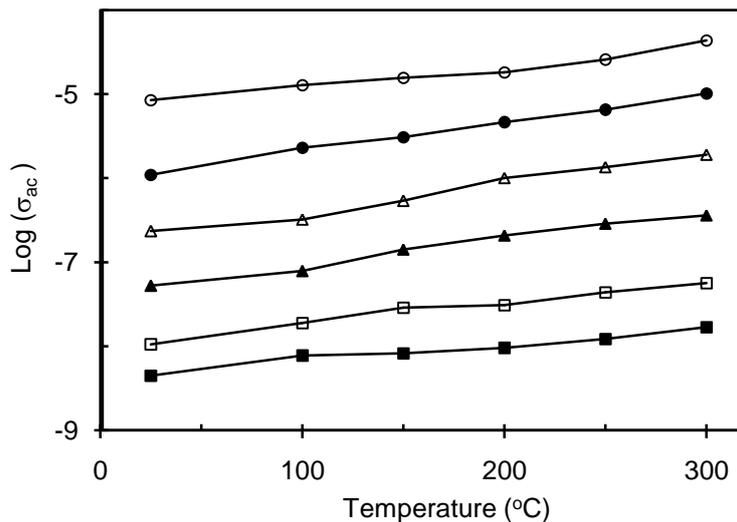
**Fig. 2:** Temperature dependence ac conductivity as a function of frequencies of ; (■) 60 Hz, (□) 330 Hz, (▲) 3 KHz, (Δ) 30 KHz, (●) 0.3 MHz and (○) 3 MHz for zirconium dioxide.
